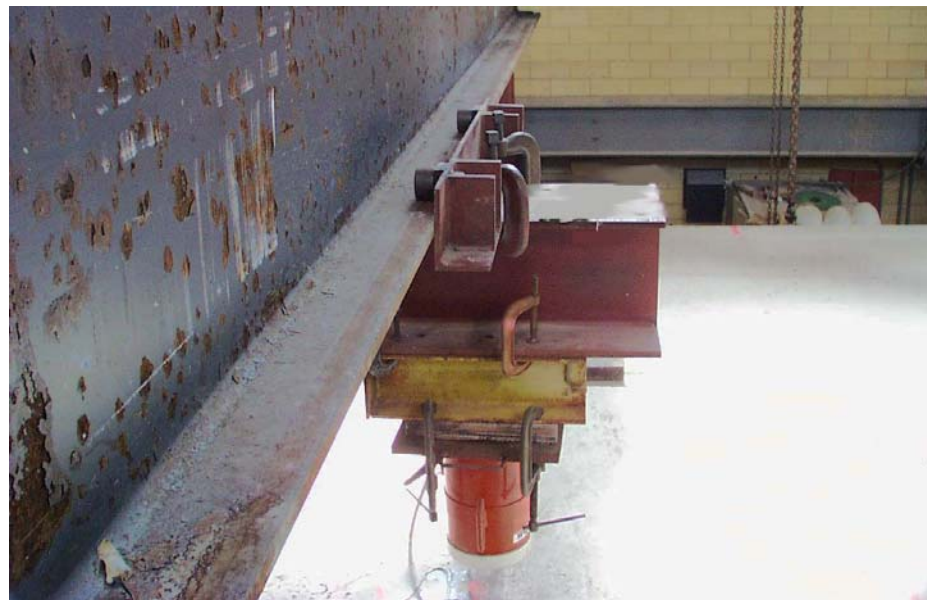
Figure 6.17 Roller attachment of actuators to load frame
