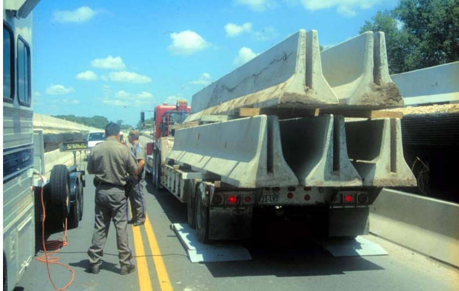
Figure 5.21 Portable scales used to weigh truck
